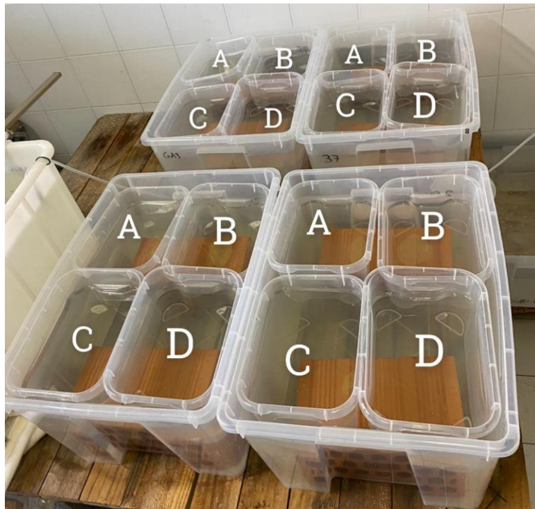
Figure 5 the picture shows the experiment set up of the 16 collection tanks in the cold condition (18°C); each larger reservoir tank contained 4 smaller tanks inside labeled A,B,C, and D based on the salinity conditions. This experimental design was also repeated in a warm room for the 28°C tanks and the 32°C tanks. The 32°C tanks contained an aquarium heater in between the two suspension bricks in the bottom of the reservoir tank to increase the temperature
