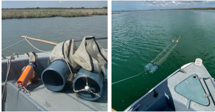
Figure 4 The picture on the left shows an up close view of the opening of the bongo net with flowmeter in the mouth of the 300 \mu m net, the bongo net is folded over the side of the boat and the wooden suspension pole to also show both ends of the net including the orange plastic containment unit at the bottom for which the catches aggregated. The picture on the right depicts the bongo net being trawled off the bow of the boat while idling backwards for collection of target species M. leidy .
