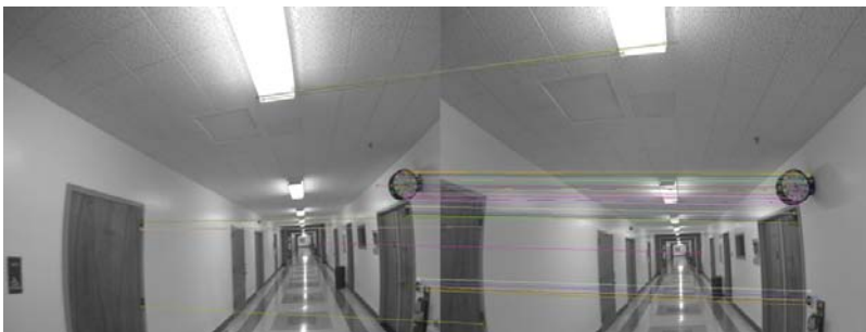
Figure 20: Matches of features extracted from a couple of time and space near frames.
