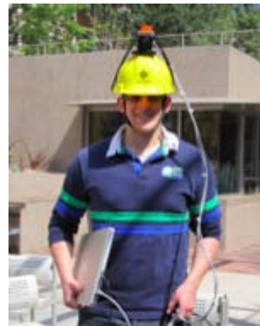
(d) Non-robot configuration. An IMU-camera system on the hardhat of an operator.
