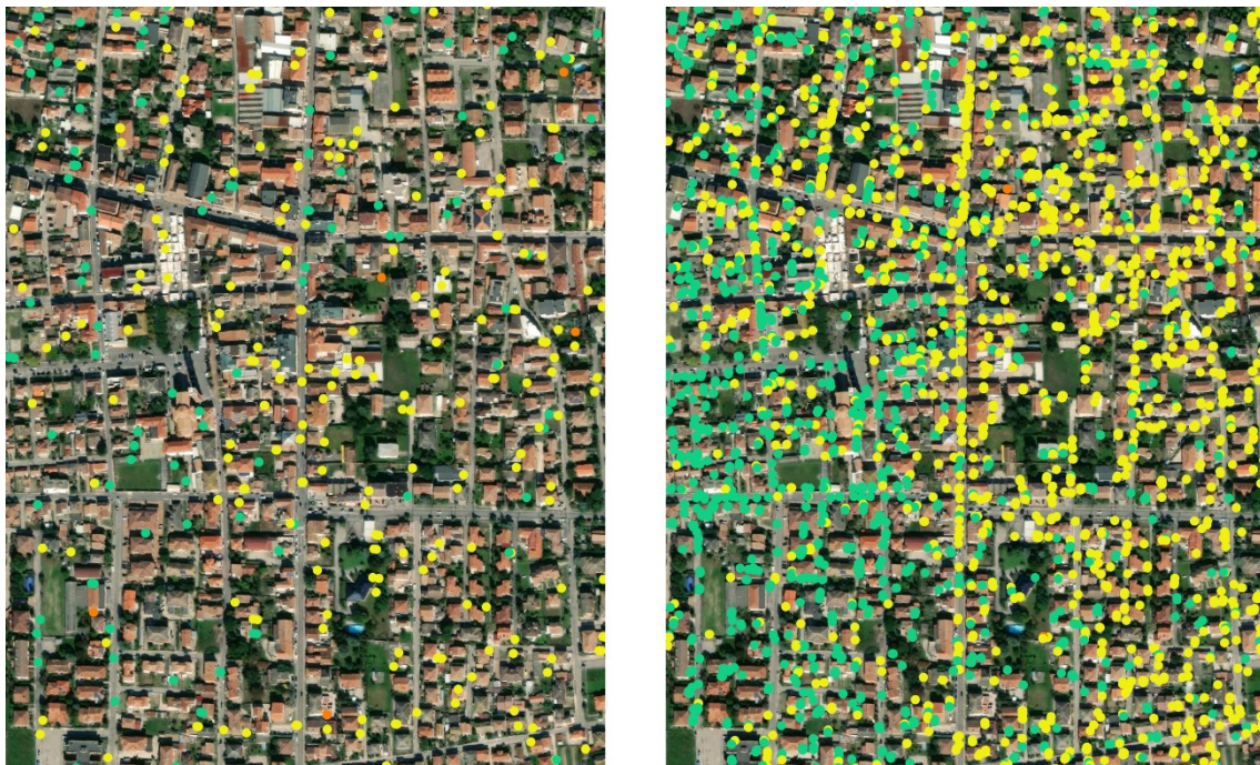
Figure 35. Difference in point density between Sentinel's and Cosmo's sensor
