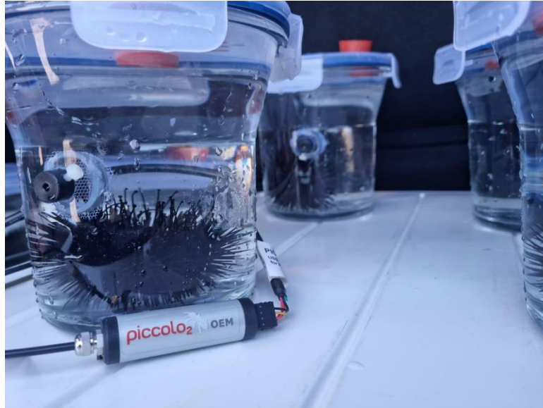
Figure 10. Image of an individual of P. lividus inside the respirometric chamber. The chambers were hermetically closed through the use of an o-ring. In front of the chambers, the Fiber-Optic Oxygen Meter Piccolo2.
