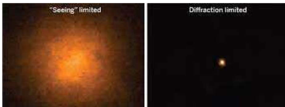
Figure 1.3: Comparison of the same image with two different systems, on the left using a seeing limited system and on the right side with a diffraction limited system, (5).
