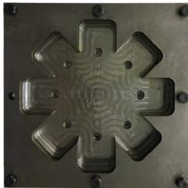
Figure 79. Clamp design for 0°, 45° and 90° sample milling
