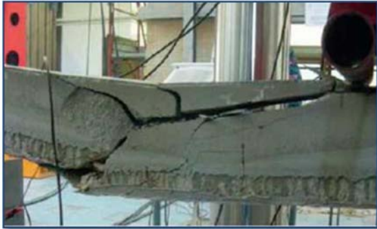
Figure 2.8 – Failure mode of beam strengthened with steel fabric [13]
