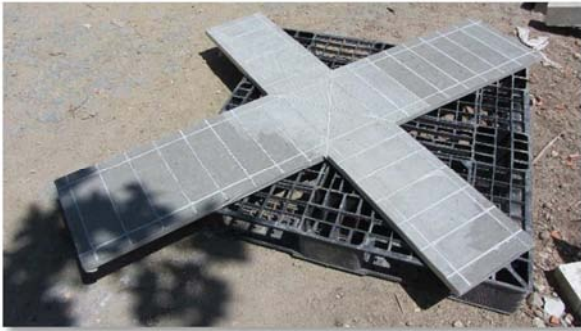
Figure 3.23 – surface not completely roughened
