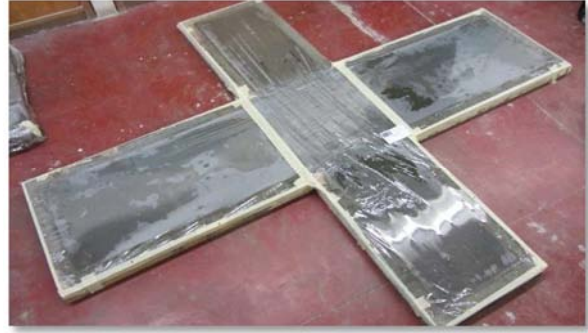
Figure 3.18 - Curing conditions of precast panels
