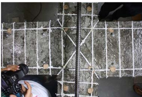
Figure 4.16 – Crack on the top surface, JPA-3
