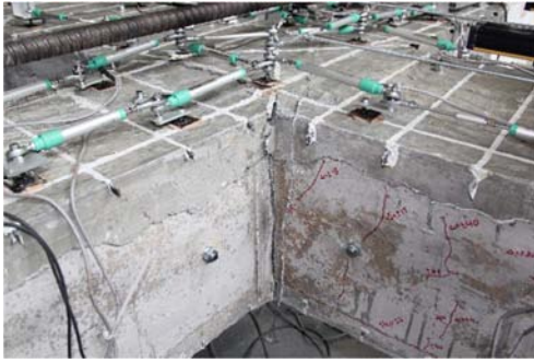
Figure 4.18 – Crack on the lateral surface, JPA-3
