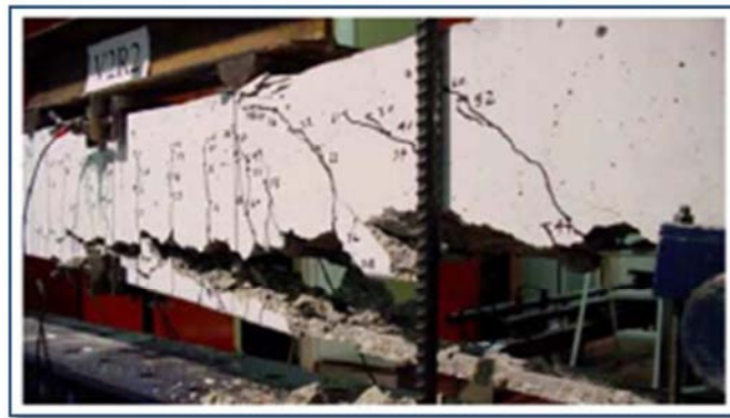
Figure 2.14 – NSM system, detachment of concrete layer [16]
