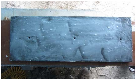
Figure 3.59 – Spreading of epoxy glue on the carbon sheet
