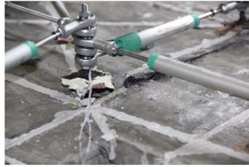
Figure 4.19 – Failure of the longitudinal bars, JPA-3
