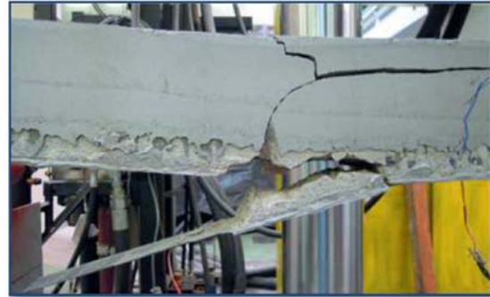
Figure 2.9 - brittle failure mode due to epoxy-concrete debonded [13]
