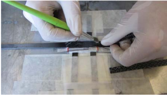
Figure 3.32 – fibers glued on laminate for a length of 5cm, red lines mark the borders
