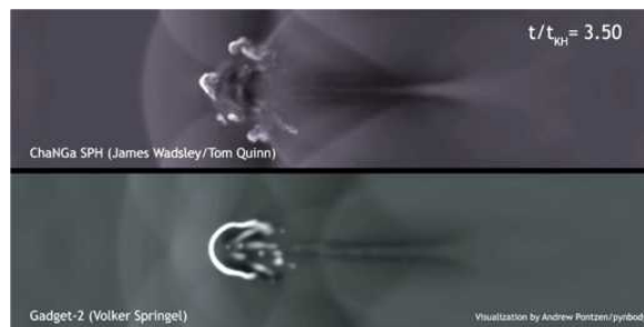
Figure 2.4: Example of gas physics simulation using ChaNGa (top panel) compared to another SPH hydrodynamic code GADGET-2 (bottom panel). The simulation is of a high dense region of gas under the influence of an external wind. The ChaNGa code shows better treatment of instabilities rapidly mixing the high density region with the surrounding medium. Time is shown in units of the Kelvin-Helmholz growth time.
