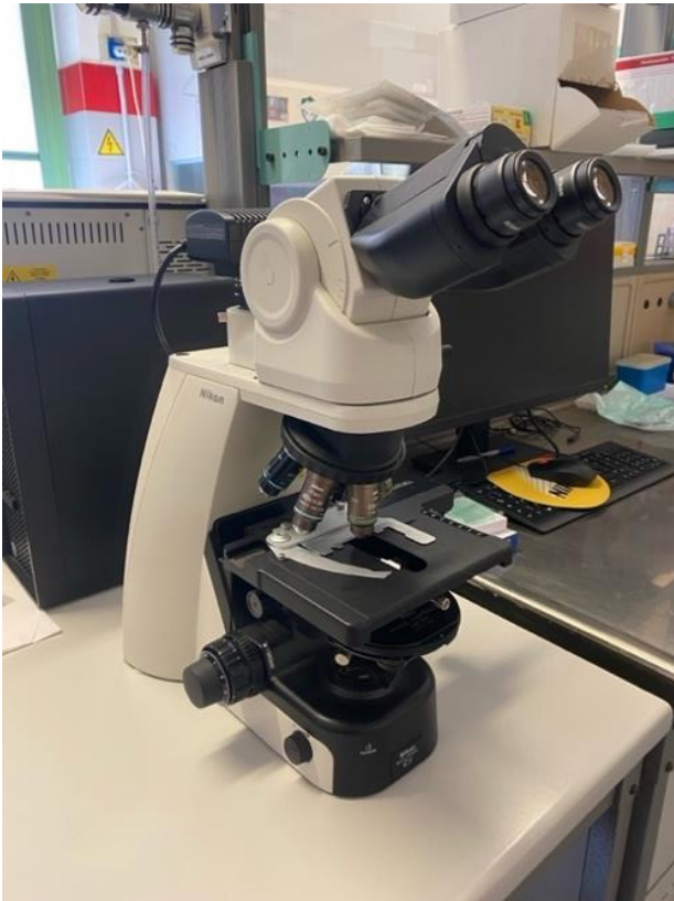
Figure 13: Light microscope (Eclipse CiTM, Nikon, Tokyo) used for vaginal smear's observation in the VTH of Padova.
