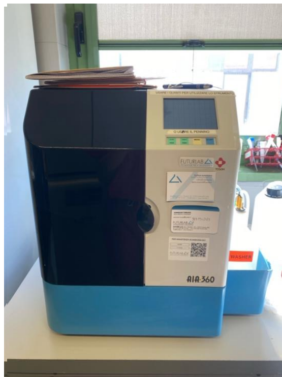
Figure 15: Automated Immunoassay Analyser-360TM, Tosoh, Tokyo used for P4 assay at the VTH of Padova
