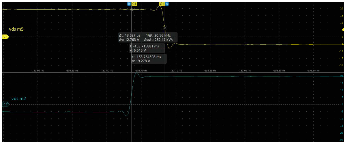
Figure 4.21: Gate signal sampled on the PCB board with an oscilloscope. The BH signal is coming from the right leg and AH from the left leg of the circuit
