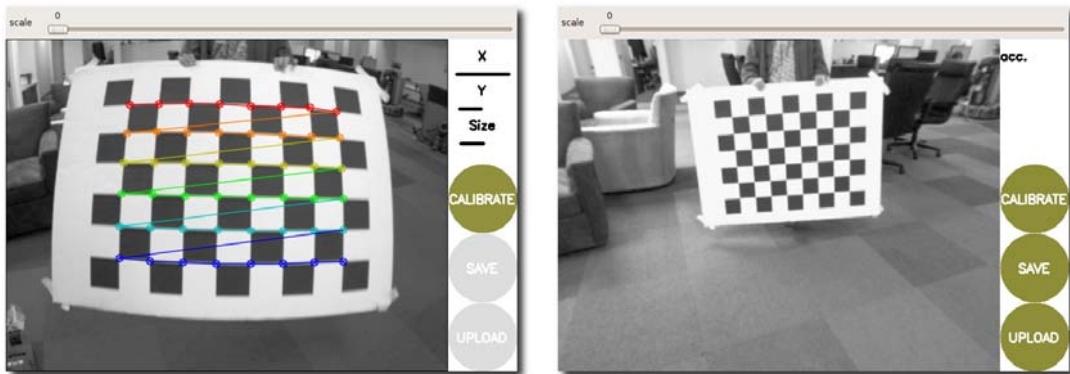
(a) A chessboard during the calibration (b) A chessboard after the calibration
