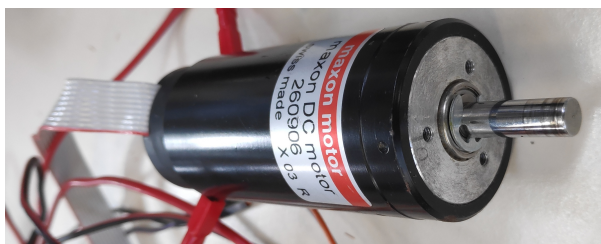
Figura 4.4: Maxon DC motor 260906.
