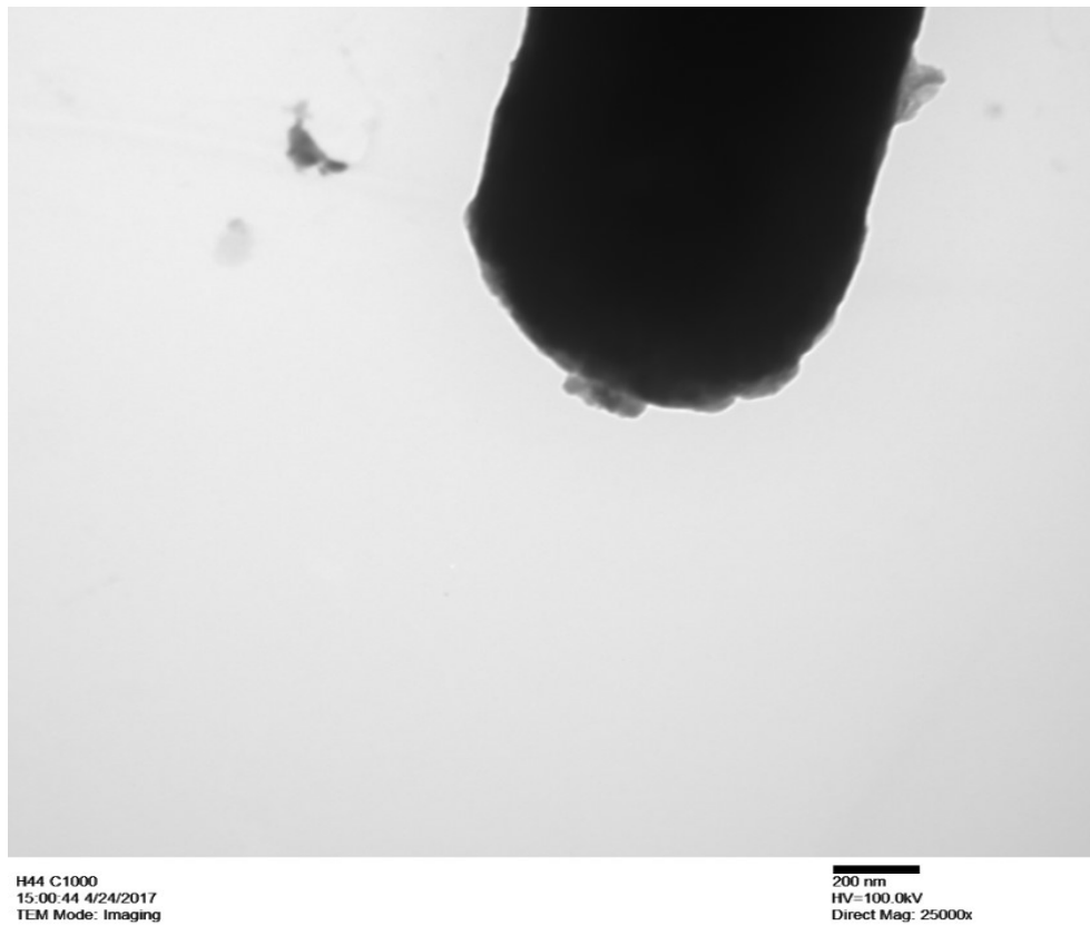
Fig. 4.1.16. The figure shows TEM Picture of H44 ceramic fiber (low mag.). (source: experimental figure)
