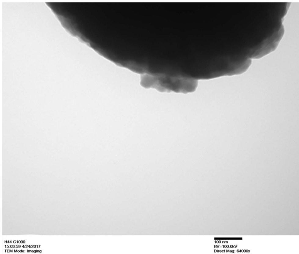
Fig. 4.1.16. The figure shows TEM Picture of H44 ceramic fiber (hig. mag.). (source: experimental figure)
