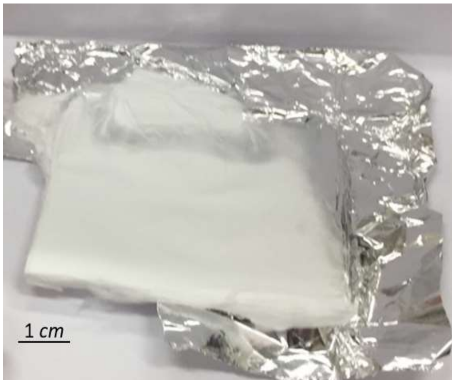
Fig. 3.1.4. The figure shows an aluminum foil with a fibrous mat (width 8 cm and height 8 cm). (source: experimental figure)
