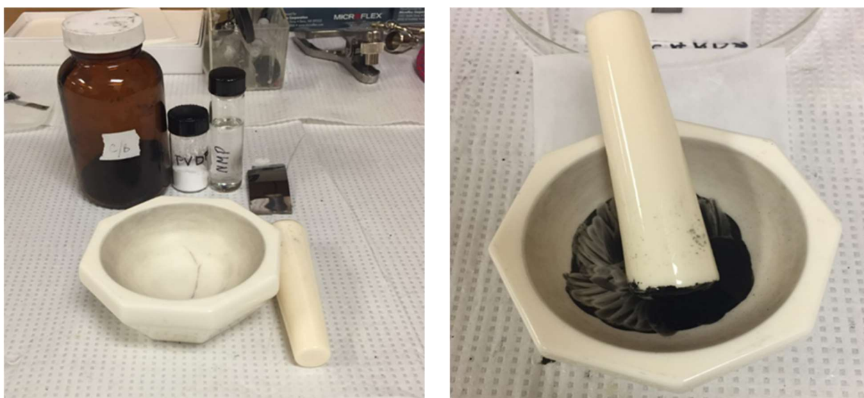
Fig. 3.5.2. The figure shows the chemicals needed for electrode preparation and the black slurry. (source: experimental figure)
