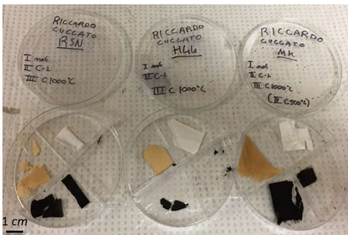
Fig. 4.1.2. The figure shows chromatic changes of the three PDCs. (source: experimental figure)
