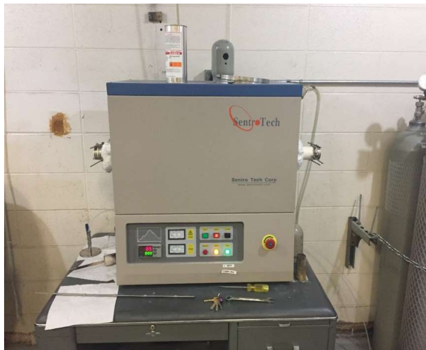
Fig. 3.2.5. The figure shows the furnace used for the pyrolysis (source: experimental figure)
