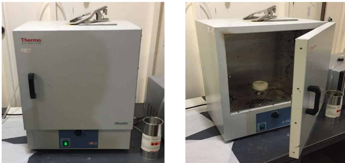
Fig. 3.2.4. The figure shows the oven used for the cross-linking (source: experimental figure)
