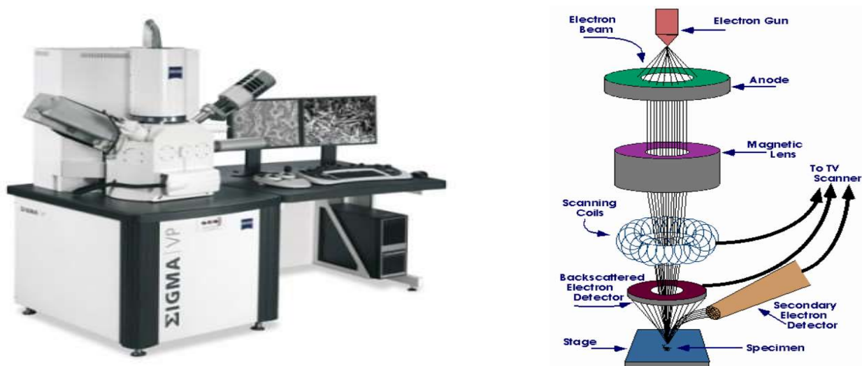
Fig. 3.4.1. The figure shows the SEM used, on the left and a scheme of a generic SEM, on the right (source: experimental figure, www.enfo.agt.bme.hu )
