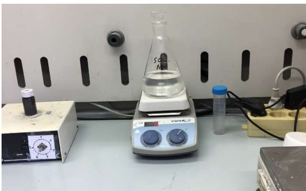
Fig. 3.1.1. The figure shows the stirring of a spinning solution. (source: experimental figure)
