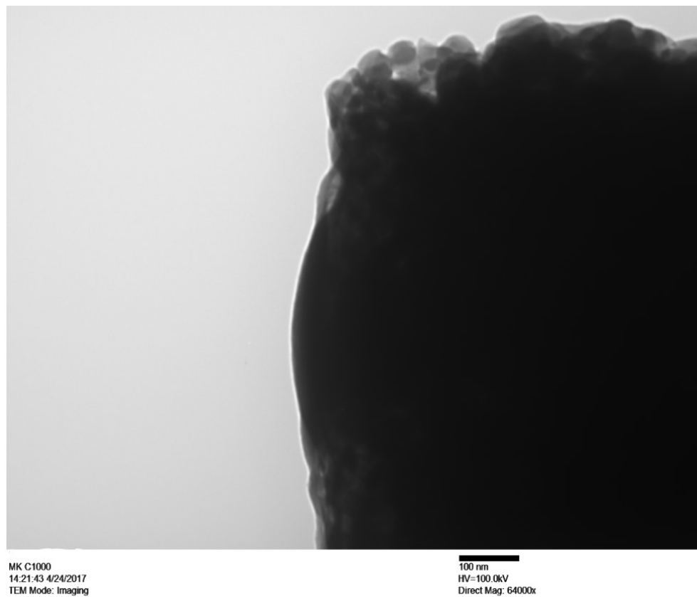
Fig. 4.1.15. The figure shows TEM Picture of MK ceramic fiber (hig. mag.). (source: experimental figure)
