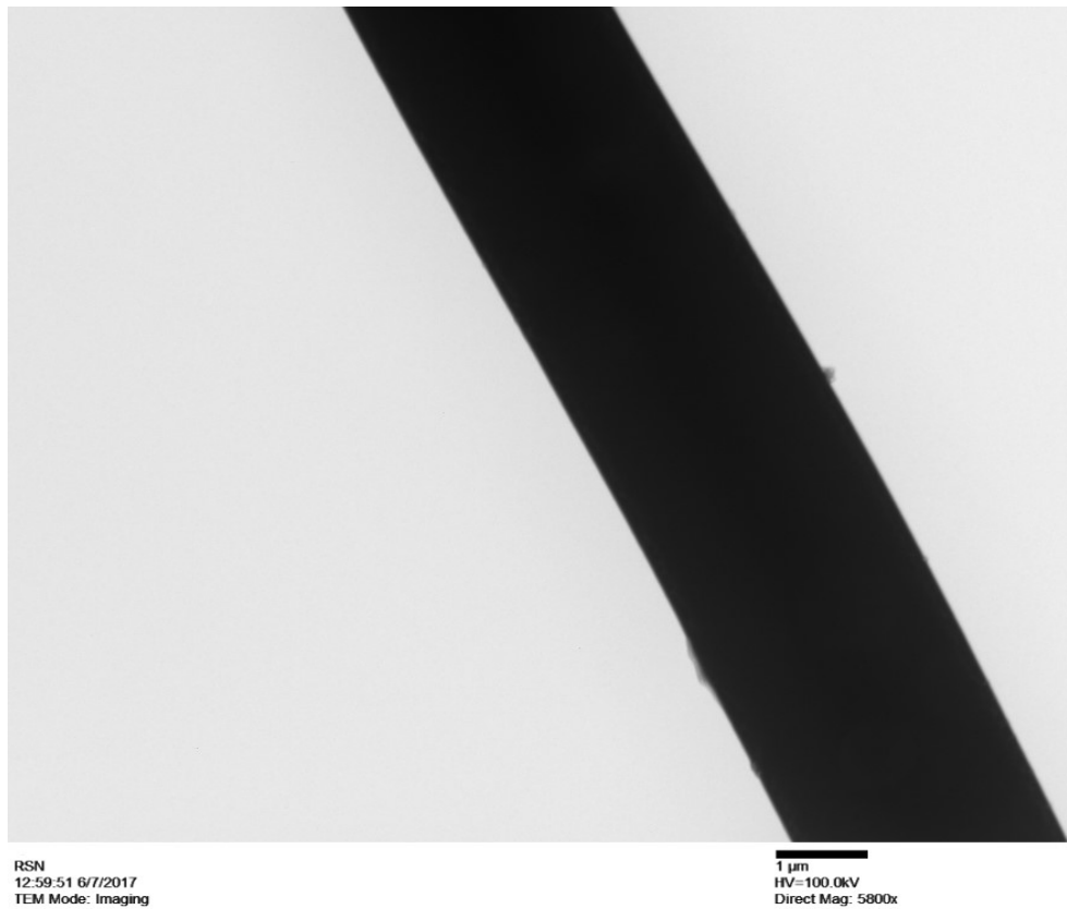
Fig. 4.1.17. The figure shows TEM Picture of RSN ceramic fiber (low mag.). (source: experimental figure)
