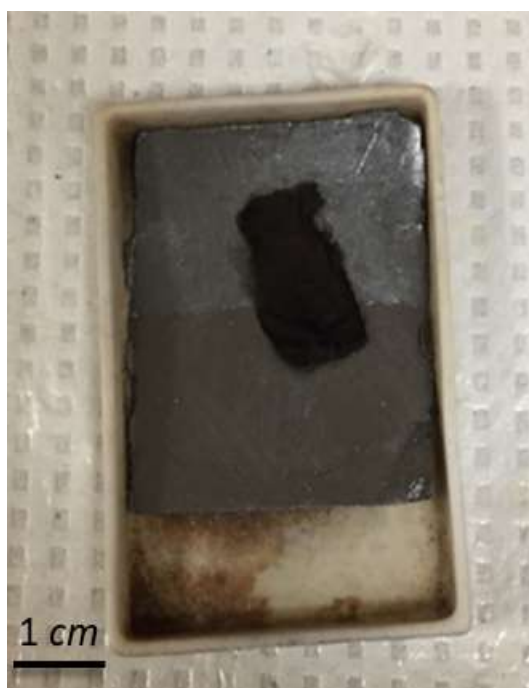
Fig. 3.2.8. The figure shows a ceramic fiber mats (dimensions of the pyrolyzed pieces: width 2 cm and height 1 cm, approximately) (source: experimental figure)
