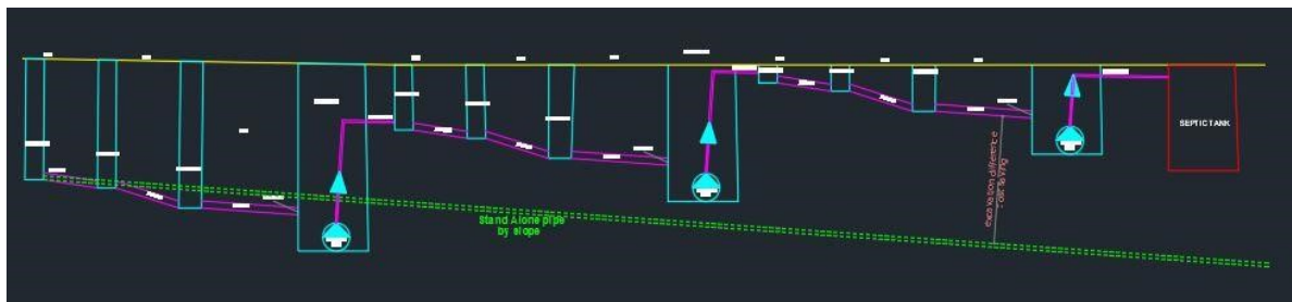
Figure 11 multi lifting stations
