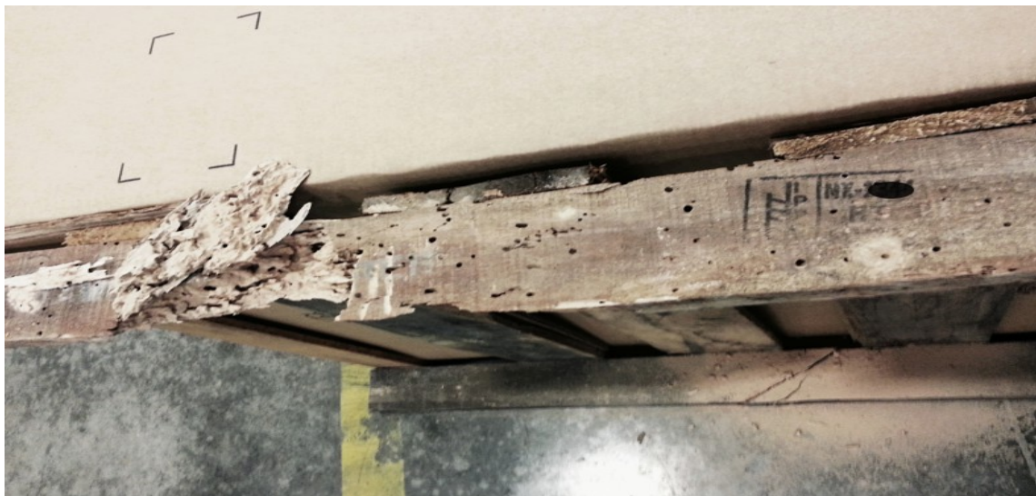
Fig. 14: Phytosanitary visual inspections verify the ISPM 15 mark and the possible presence of holes or sawdust indicating the presence of alive insects
