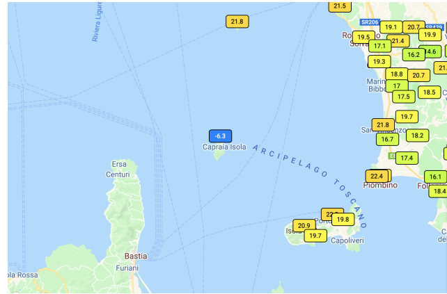
(b) Example of bad data detected by the difference between model and stations.
