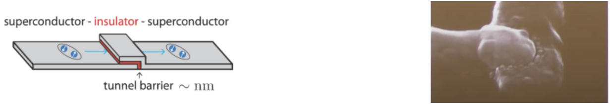
Figure 3.6: On the right a scheme of a Josephson junction composed of SC-insulator-SC, with the cooper pairs tunneling. On the left a microscope image of a JJ.
