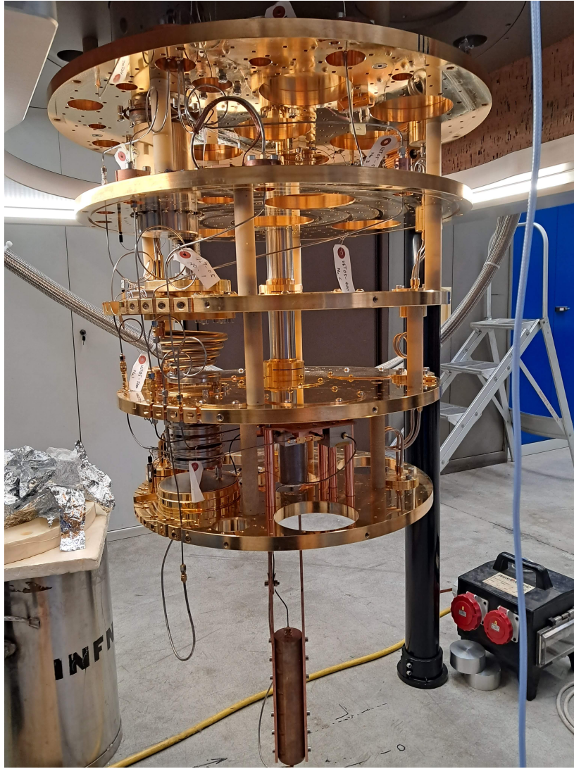
Figure 4.7: Photo of the DR equipped with all the elements of the present experiment.
