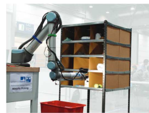
(b) Image taken from [22] of an UR10 arm with a Kinect V2 RGB-D camera on its end-effector, used for picking object task.
