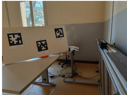
Figure 5.9: Image of the complete setup used in Depth Accuracy benchmark. It can be seen that in distances less than 2.5m it is used a desk as a support for the plane given its height less than 0.5m.
