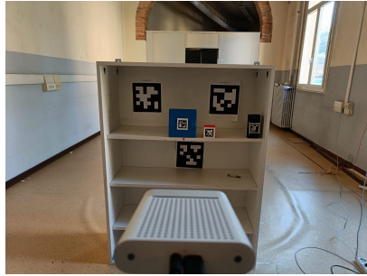
(a) Image of Depth Contour benchmark representing: cabinet with its 3 AprilTag that will define the plane, and 3 basic object with its AprilTag for object detection.
