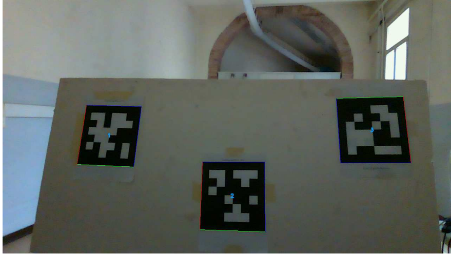
Figure 5.4: Example of the image published in topic /tag_detections_image . This topic is used just for a check that the AprilTags are detected correctly inside the image.
