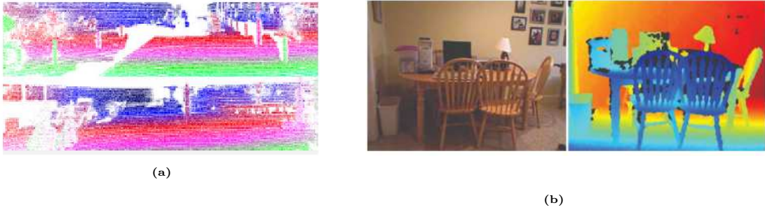
Figure 2.8: Example of Real-dataset:(a) sparse depth from KITTI Depth Completion Benchmark (b) depth from NYU-v2 dataset
