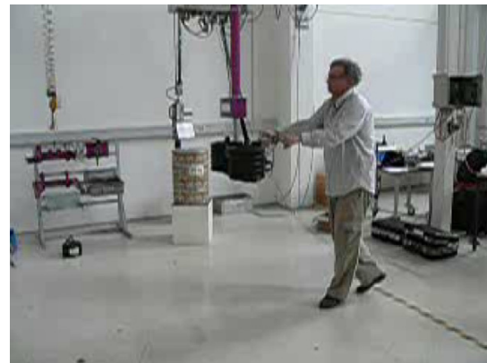
(b) Rail crane based cobotic system providing power supply in order to reduce apparent inertia of heavy workpieces (Surdilovic D et al. 2005, 2007).
