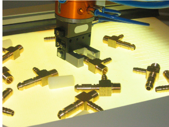
Figura 3.26: Camera equipped belt feeder for feeding and picking arbitrarily oriented components.
