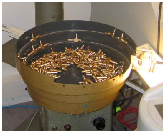
Figura 3.25: Vibratory bowl feeder with active sensing reorientation. The vision system identifies the component for pick up. Unsuitably positioned components are returned to the bowl by a pneumatic pusher.
