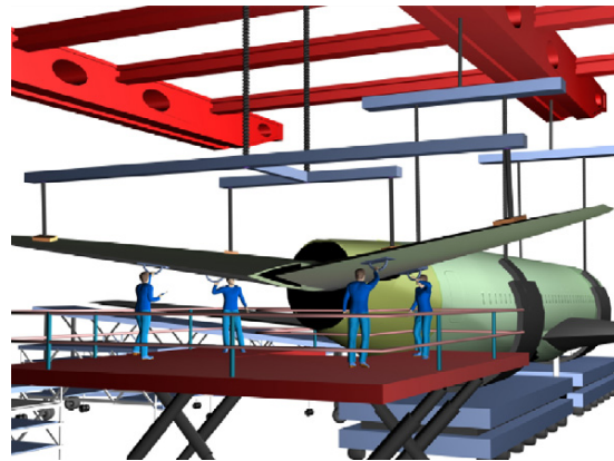
Figura 3.35: Application of cobotic devices in future human-robot-human interaction for airplane assembly (Krüger J et al. 2008).
