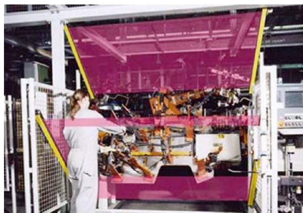
Figura 3.15: Application of active opto-electronic protection devices in assembly.
