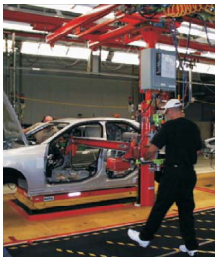
Figura 3.3: Cockpit install with IAD ( www.stanleyassembly.com ).
