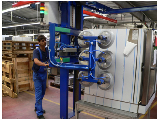
Figura 3.34: First admittance display prototype in industry (Krüger J et al. 2006).
