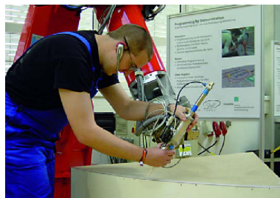
(b) Teaching the robot by manual guidance using force-torque-sensors.
