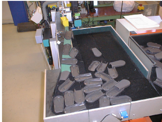
Figura 3.24: Vibratory brush feeder for gentle feeding of fragile parts.
