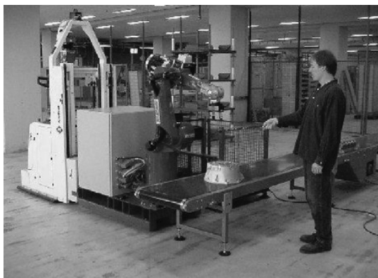
(a) The worker is pointing out objects directly in the scene using a laser pointer (Stopp A, Horstmann S, Kristensen S, Lohnert F, 2003).
