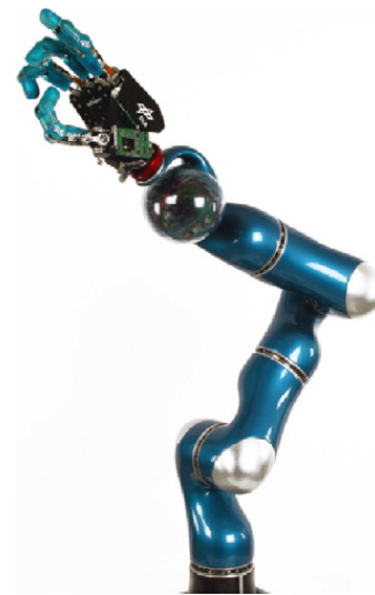
(b) Humanoid light weight robot structure (Albu-Schäffer A et al. 2007).
