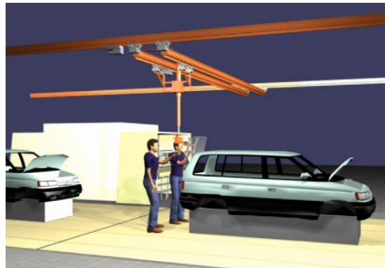
Figura 3.29: Cobotic system for feeding and positioning of large assembly parts.
