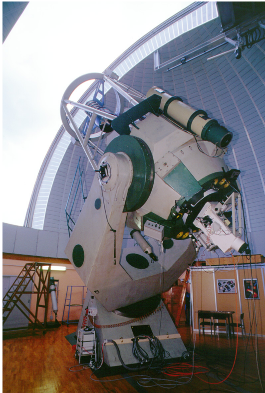
Figure 2.6: The 182 cm 'Copernico' telescope at Cima Ekar (Asiago, VI).
