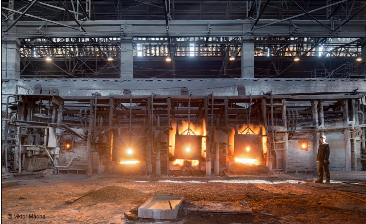
Figure 1.3. B-stall, 60-ton open-hearth furnace (viktormarsha.com,2022)
