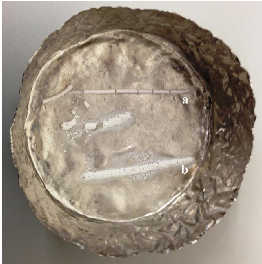
Figure 36. (a) MK + 58.3% \text{CaCO}_3 and (b) MK + 52.5% \text{CaCO}_3 + 10% wax rods after pyrolysis
