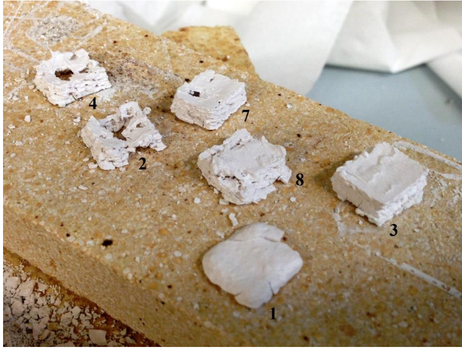
Figure 60. Pyrolyzed ceramic parallelepipeds
