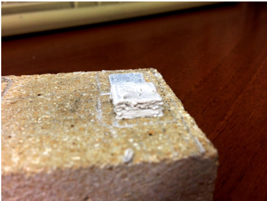
Figure 58. Printed preceramic parallelepiped
