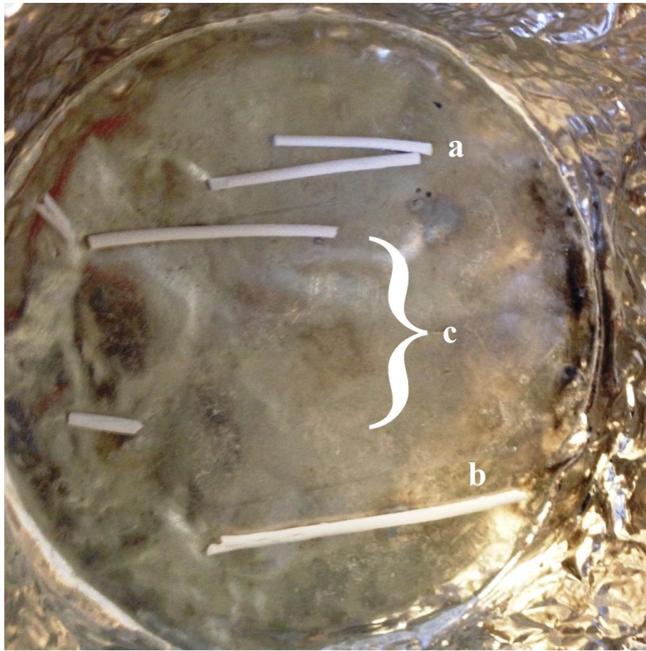
Figure 41. (a) MK + 58.3% \text{CaCO}_3 , (b) MK + 52.5% \text{CaCO}_3 + 10% wax and (c) MK + 56.6% \text{CaCO}_3 + 3% wax rods after pyrolysis with 1^\circ\text{C}/\text{min} heat rate
