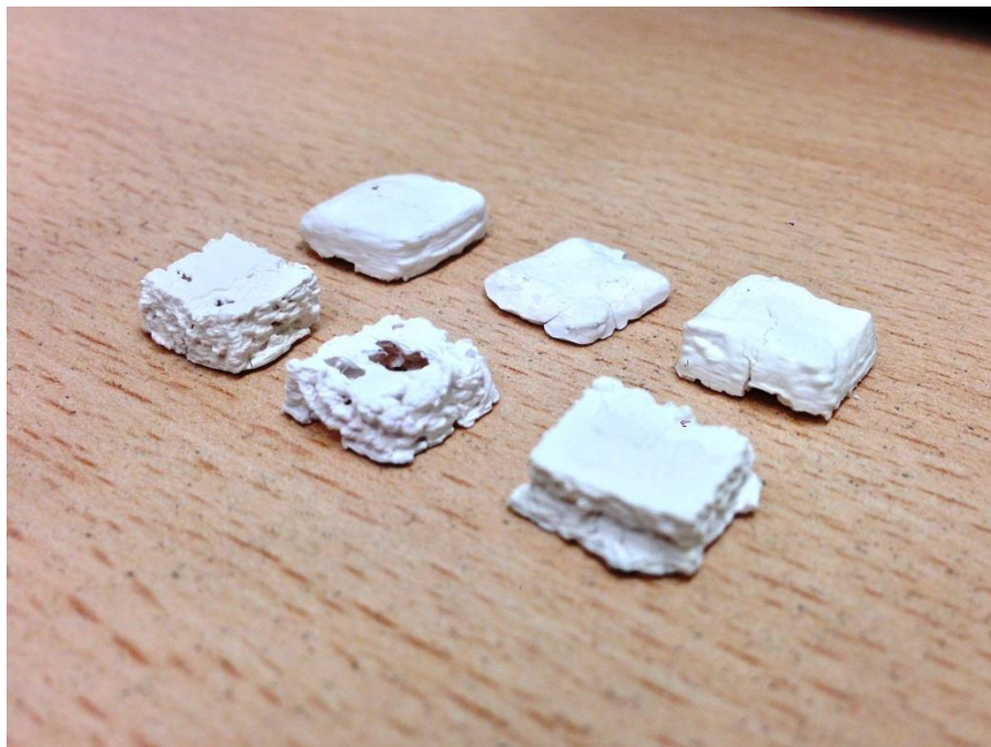
Figure 62. Ceramic printed samples after immersion in SBF solution
