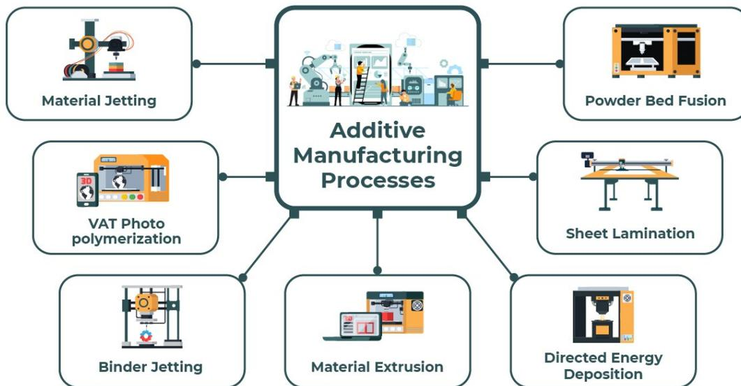
Figura 8: Tecniche di Additive Manufacturing (Kambale, 2021)
