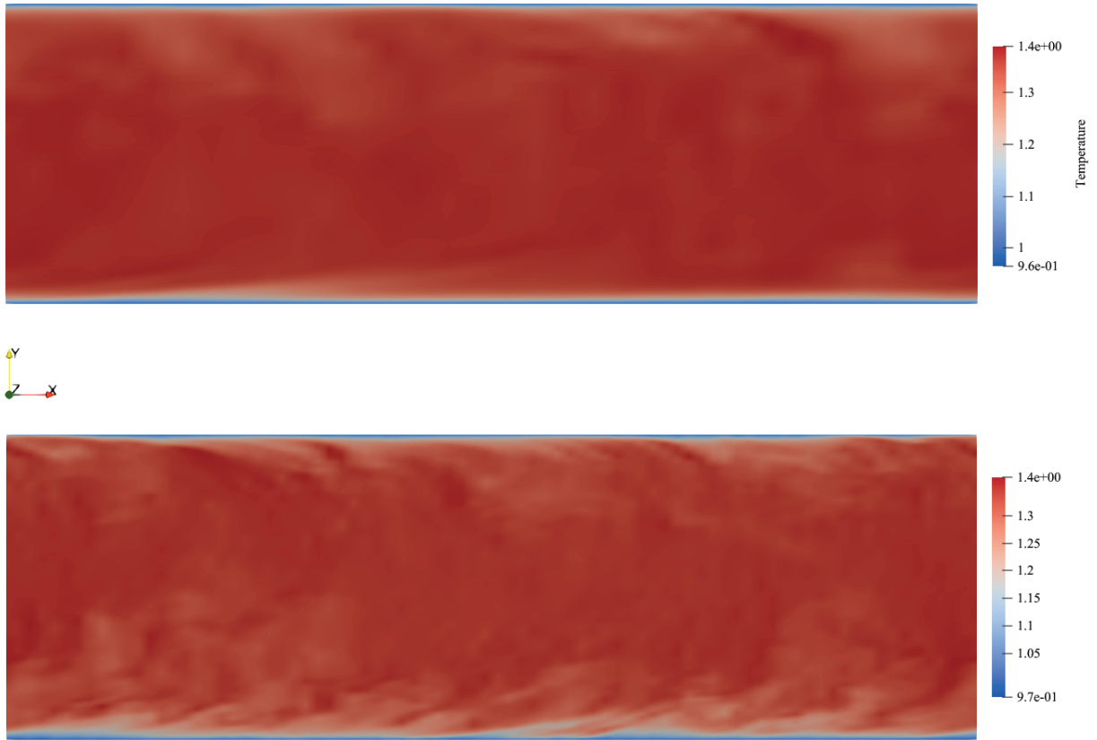
Figure 6.15: z -normal slice of the temperature fields at the side of the channel at M_\infty = 1.5 and Re_\tau = 215 (top) and Re_\tau = 500 (bottom) using the mixed time scale (MXTS) model.
