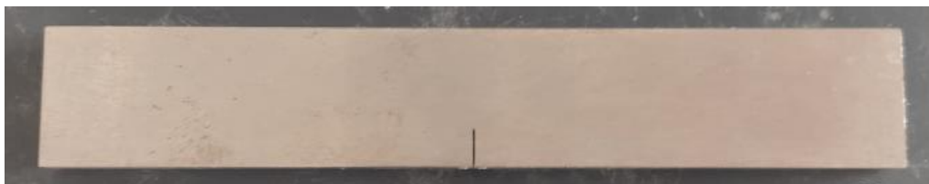
Figura 8.29: provino SENB ASM01
