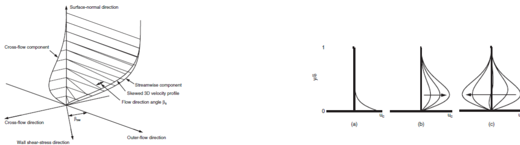
Figure 2.8: Schematic of a 3D velocity profile, and different types of cross-flow profiles: a) Shear driven cross-flow due to the motion of the wall, b) pressure driven cross-flow increasing c) pressure driven cross-flow reversing [13]
