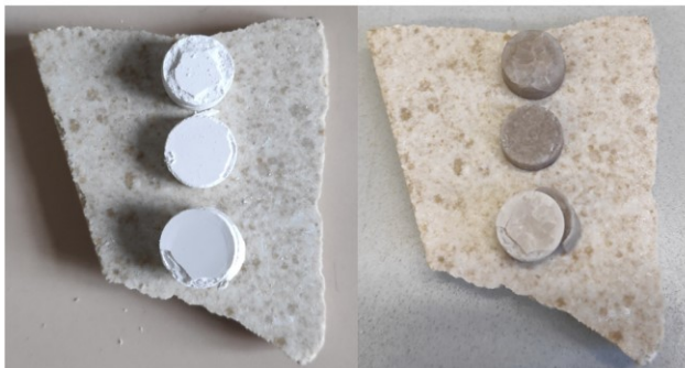
Figure 4.6: tablets before (left) and after (right) thermal treatment, in order from top to bottom 50/50 molar, 79/21 molar and 100/0 molar.
