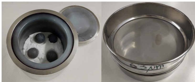
Figure 3.1: Agate jar with the powder and the Agate spheres inside on the left and the 63 micron sieve on the right.
