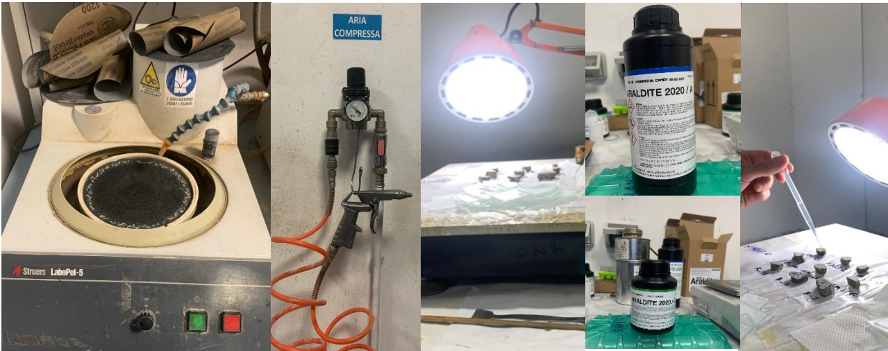
Figure 77: The Instruments used to create the thin sections for Optical Microscopy.
