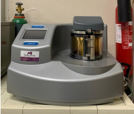
Figure 78: Quorum Q150R Rotary pump Coater used for gold coating.
