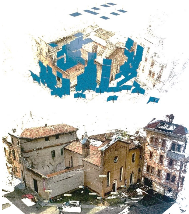
Figure 43: a photogrammetry model of Oratorio di San Michele, using a drone (Talami, 2024).
