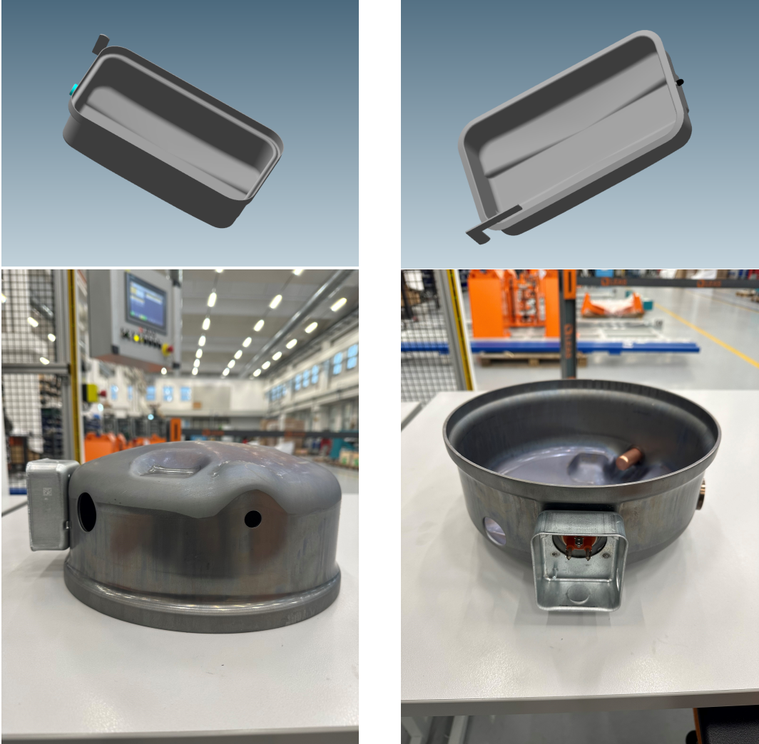
Figure 4.59: Two types of Expansion Tanks
