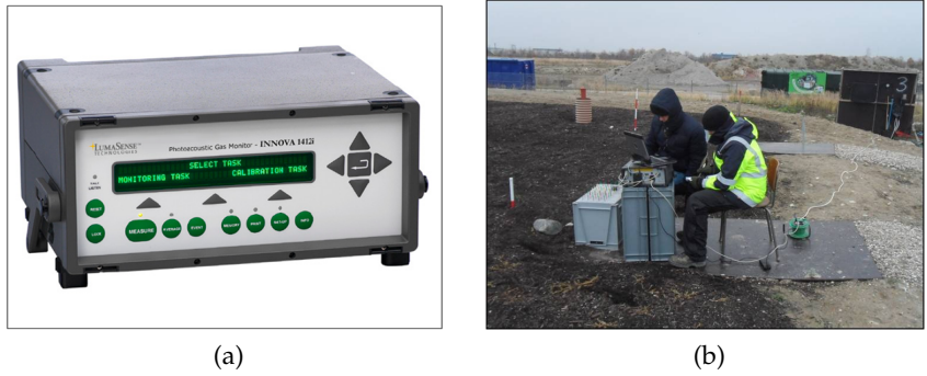
Figure 22: (a): Photoacoustic Gas Monitor INNOVA 1412i equipment (LumaSenseTechnologies, 2012), (b): INNOVA 1412i used for underground gas sampling at AV Miljø biofilter.
