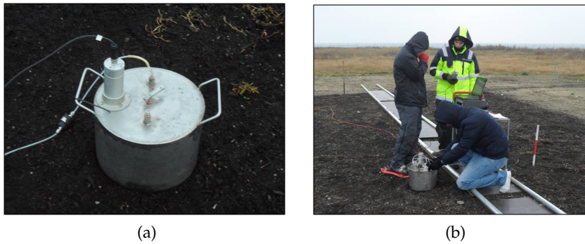
Figure 25: (a): Static flux chamber placed on the biofilter. It's possible to observe the cylindrical Vaisala probe and the tube connecting the chamber with INNOVA equipment , (b): One flux chamber test performed at AV Miljø biofilter.
