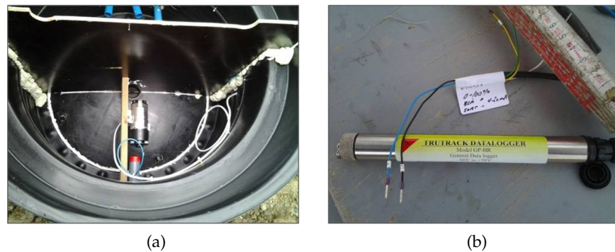
Figure 13: (a): OLCT IR gas detector placed inside the mixing chamber for methane concentration measurement, (b): GP-HR TruTrack outdoor data logger connected to the gas detector inside the mixing chamber.
