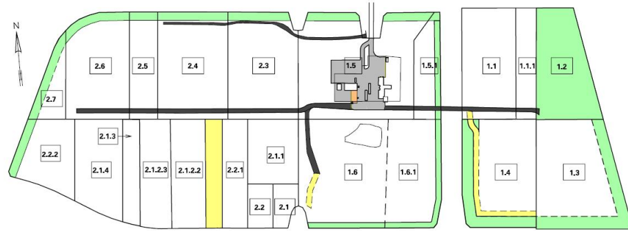
Figure 6: AV Miljø landfill plant view. Green areas represent finally top covered sectors, light gray areas represent the administration zone, yellow areas represent gravel roads, and dark gray areas represent paved roads (KøbenhavnsAMT, 2006).
