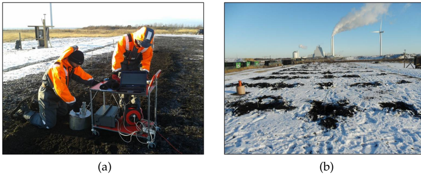
Figure 27: (a): Static flux chamber test at AV Miljø biofilter. (b): Disposition of the 60 sampling points where the flux chamber test has been performed; the snow and the frozen soil have been previously removed from the top surface in order to let flow the biogas naturally.
