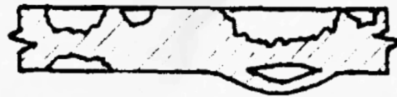
Damage Class C3: Detached spall
