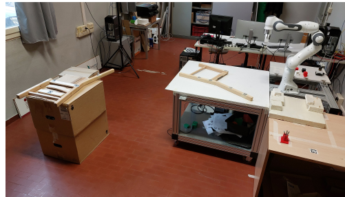
Figure 5.2: Experimental setup: in particular this is the initial situation, with one side part on the work table, other components on the left and screws in the red container on the right
