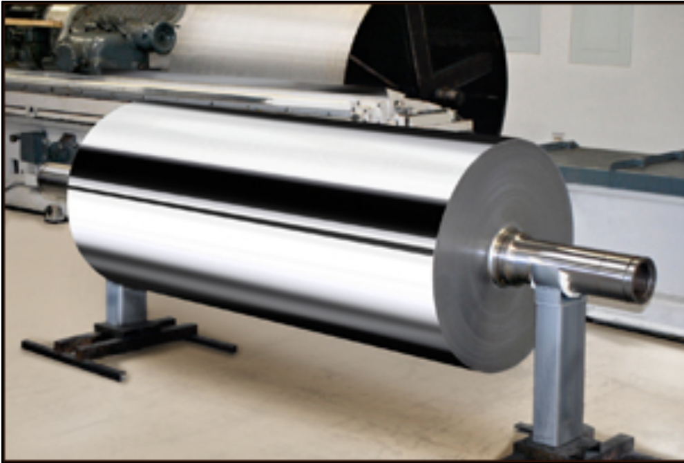
Figure 2.1 Thermo-oil heated roll [14]
