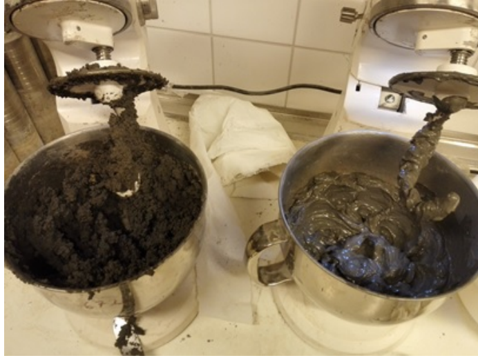
Figure 1.13: Mixing trial conducted on Dalvägen clays (courtesy of Sweco).
