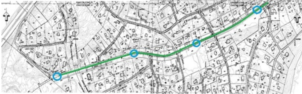
Figure 2.15: figure representing the road Dalvägen (in green) and the position of the four piezometer (blue circles).
