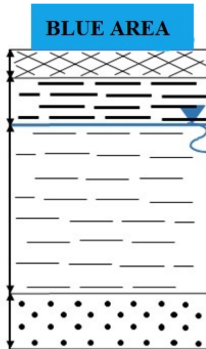
Figure 2.22: Figure representing the layering of the soil and the level of the GWT in the blue area. The thickness of the clayey layer is between 3 – 6 m .
