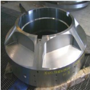
*Figura 1.9 Bearing housing*
