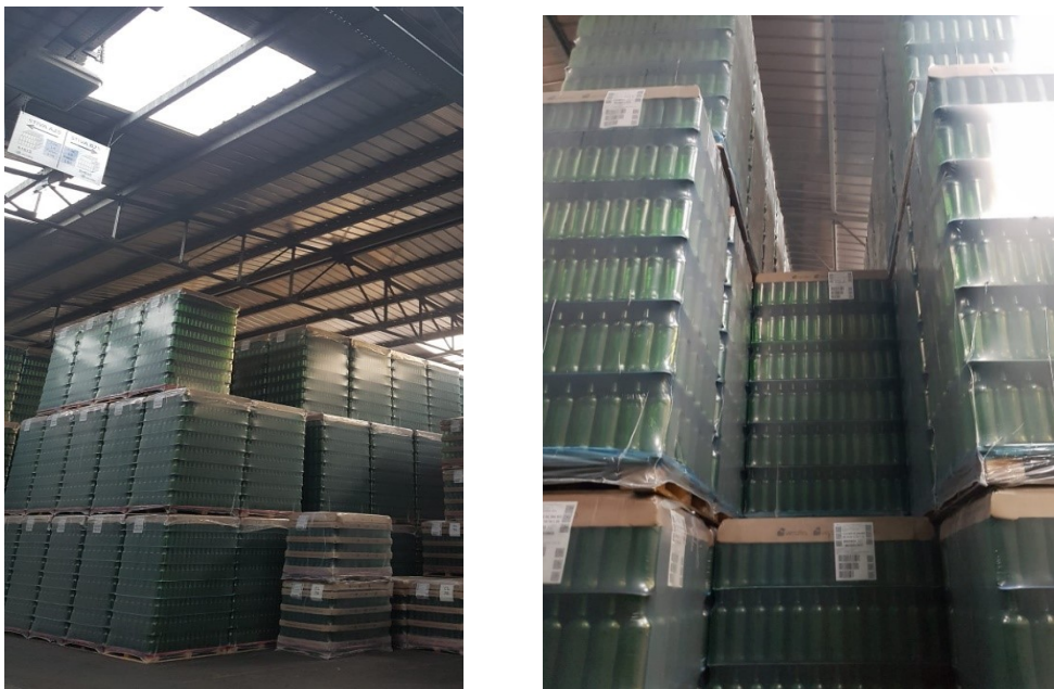
Figure 24: Pyramid structure with incomplete walls due to “Lot Separation”
