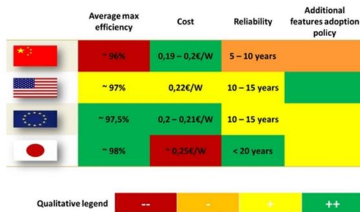
Figure 45 Inverters efficiency, cost and reliability
