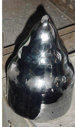
Figure 4 cylindrical section cut off to make wafers
