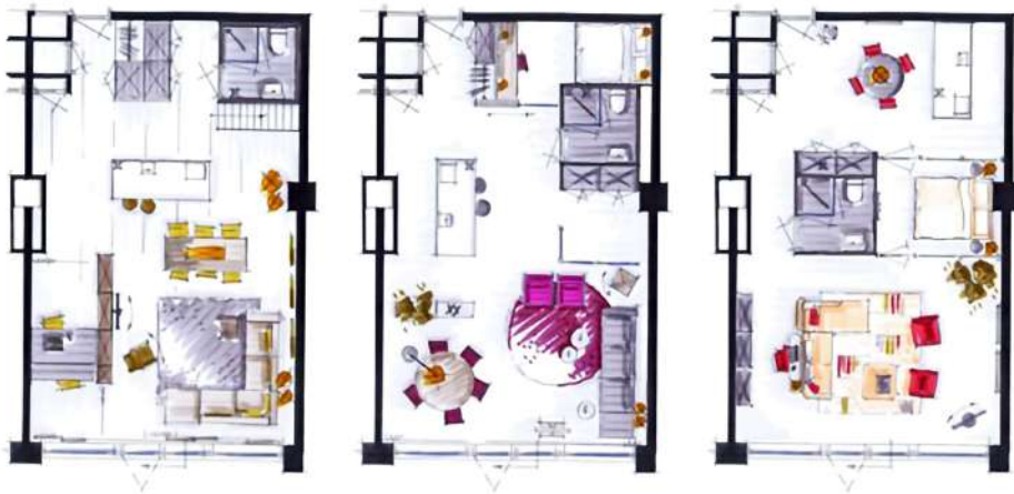
Fig.70 The units are designed to be customisable and modifiable over time. These are some of the possible flat layouts in the Hoge Rue's buildings. (Source: driehoekstriips.nl/files/25109 )
