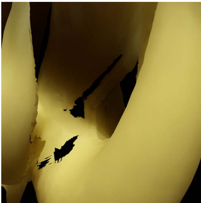
Figure 5.22: Back holes in the final appearance caused by a suboptimal placement of cameras.
