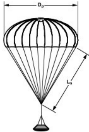
Figure 11: Supersonic parachute geometrical parameters/2
