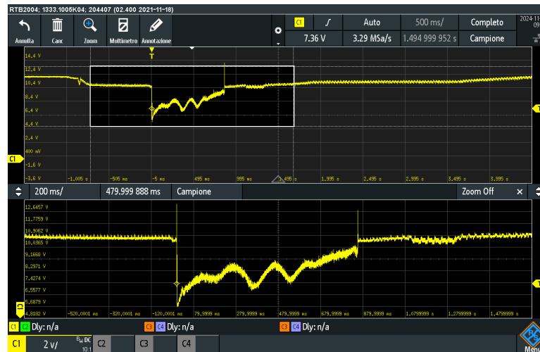
Figure 5.12: Real case: voltage cranking, diesel car
