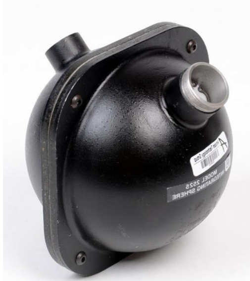
(Figure 7.9: integrating sphere)
