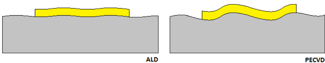
Figure 5.3: The deposition technique used (ALD or PECVD) can affect not only the thickness uniformity of the layer grown but also the effective area of the metallization.
