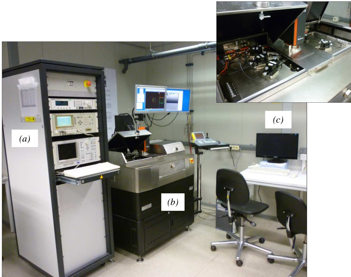
Figure 4.3: Setup for electrical measurements. All the main parts are well visible: (a) the PA300 electrical probe-station, (b) the HP4284A precision LCR-meter and (c) the computer workspace to control the measure operations.
