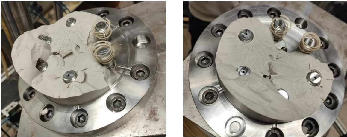
Figure 3-9: first PEEK insulator's fracture surface after rupture.
