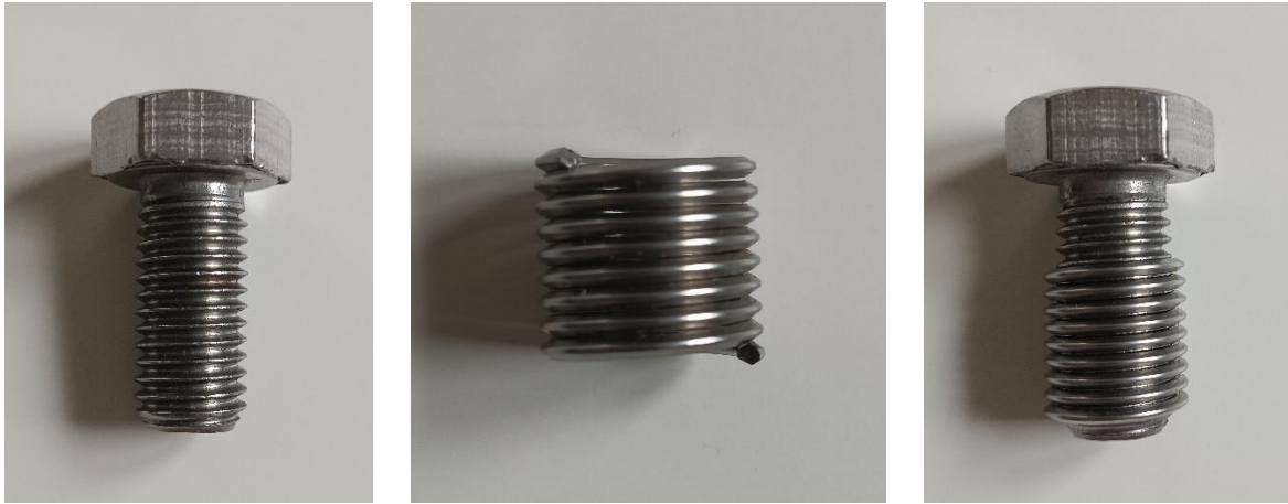
Figure 6-5: respectively from left to right: M14 screw, M14 helicoil and their assembly.
