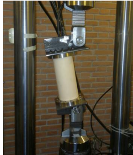
Figure 2-6: equipment sketch design (left) and insulator prototype during testing (right) 34 .
