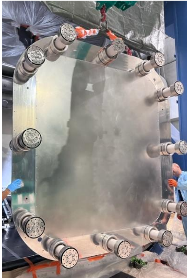
Figure 2-5: Installation of insulators on a frame of the MITICA Mock-Up Beam Source. 38
