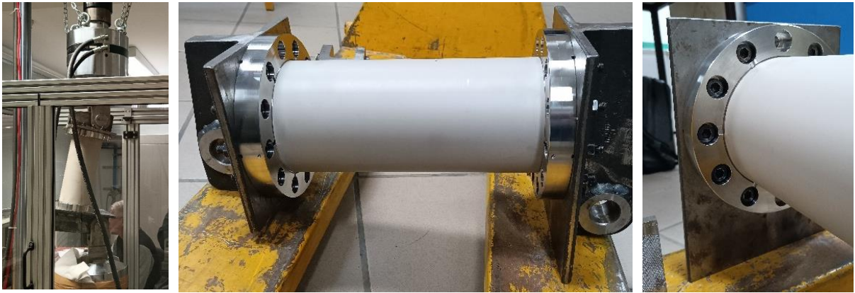
Figure 3-3: PEEK insulator assembly and testing configuration.
