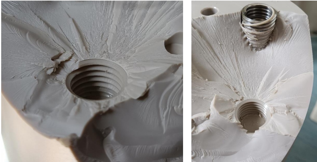
Figure 5-7: fracture at M14 helicoil and PEEK material of the fourth insulator sample.
