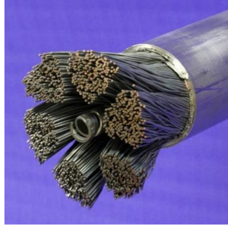
Figure 1-8: example of ITER's toroidal field conductor.
