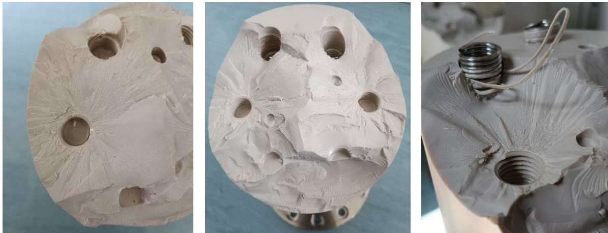
Figure 5-1: mechanical breakdown of PEEK post-insulator sample 2 (left), 3 (middle) and 4 (right).
