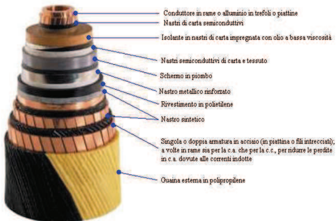
Figura 4.3 – Cavo riempito in olio SCFF
