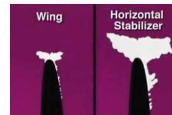
Figure 5. Typical Icing Accumulation on Leading Edges
