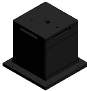
fig. 2.5: Graphite box of G2.5 configuration
