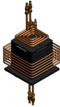
fig. 2.2: G2.5 inside: inductor and monolith box
