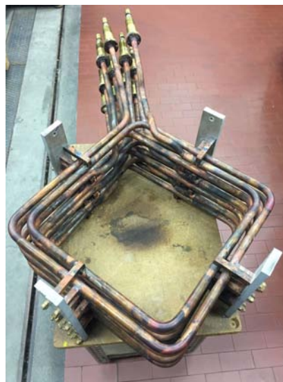
fig. 1.9: An example of linear stirrer: i DSS lateral inductor
