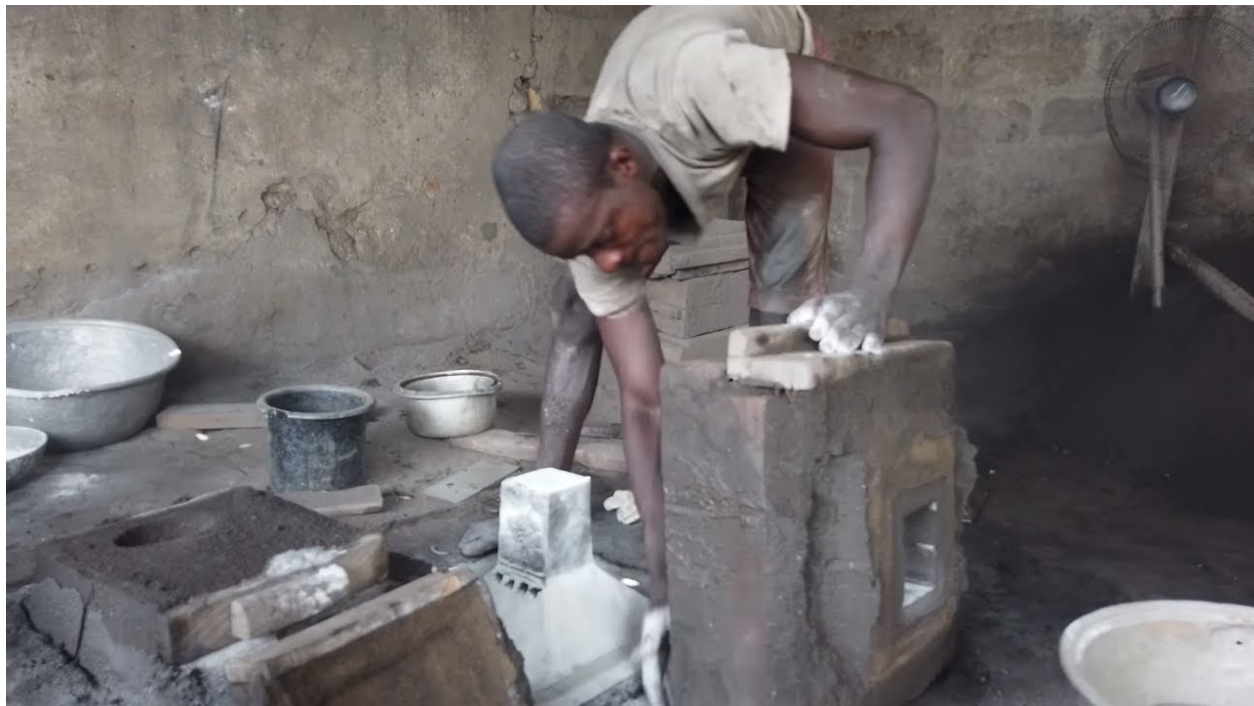
Figure 2 local artisan producing coal pot from melted metal from a discard e-waste. https://www.youtube.com/watch?v=qpGXsHJwFGE
