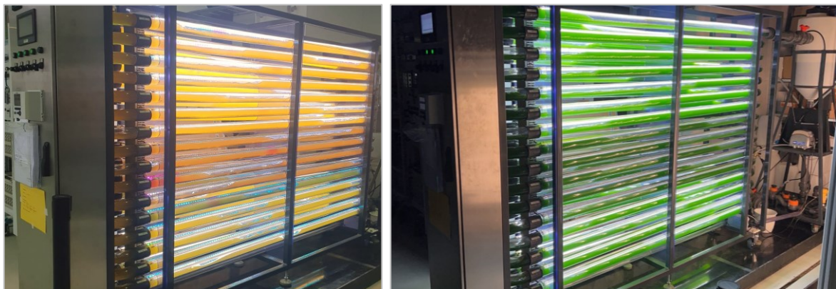
Figure 2.4. The 200L tubular reactor during the first phase (on the right) and second phase (on the left) of the operation.
