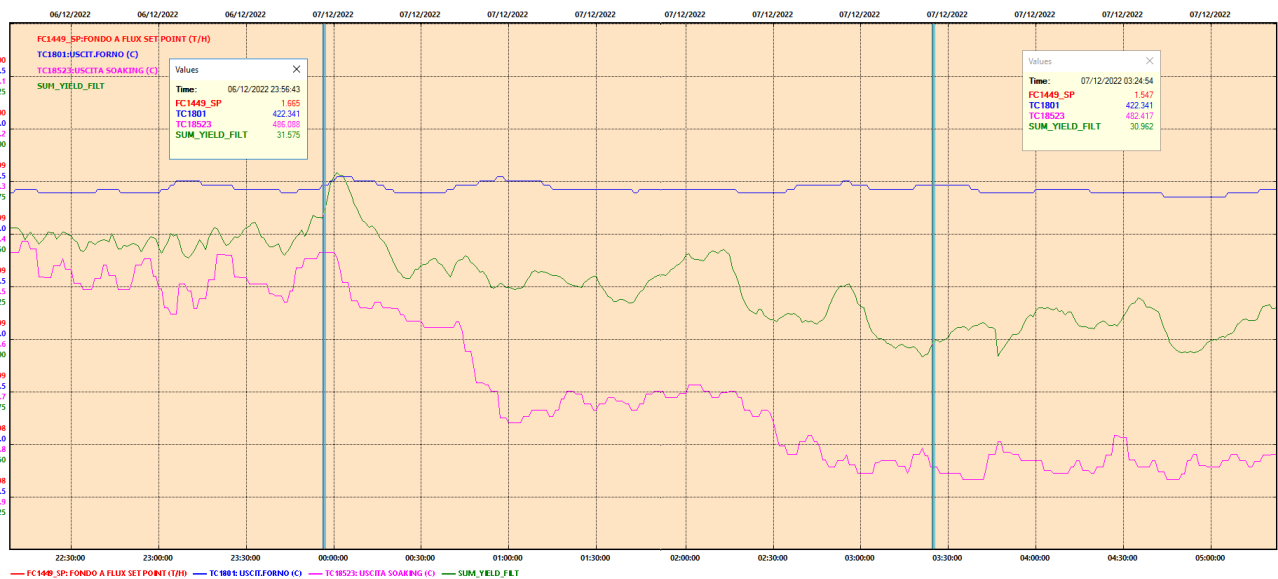
Figure 5.6 Trends of the variables of FOT and the cumulative percentage yield of distillates specifically related to thermal cracking under the same conditions.
